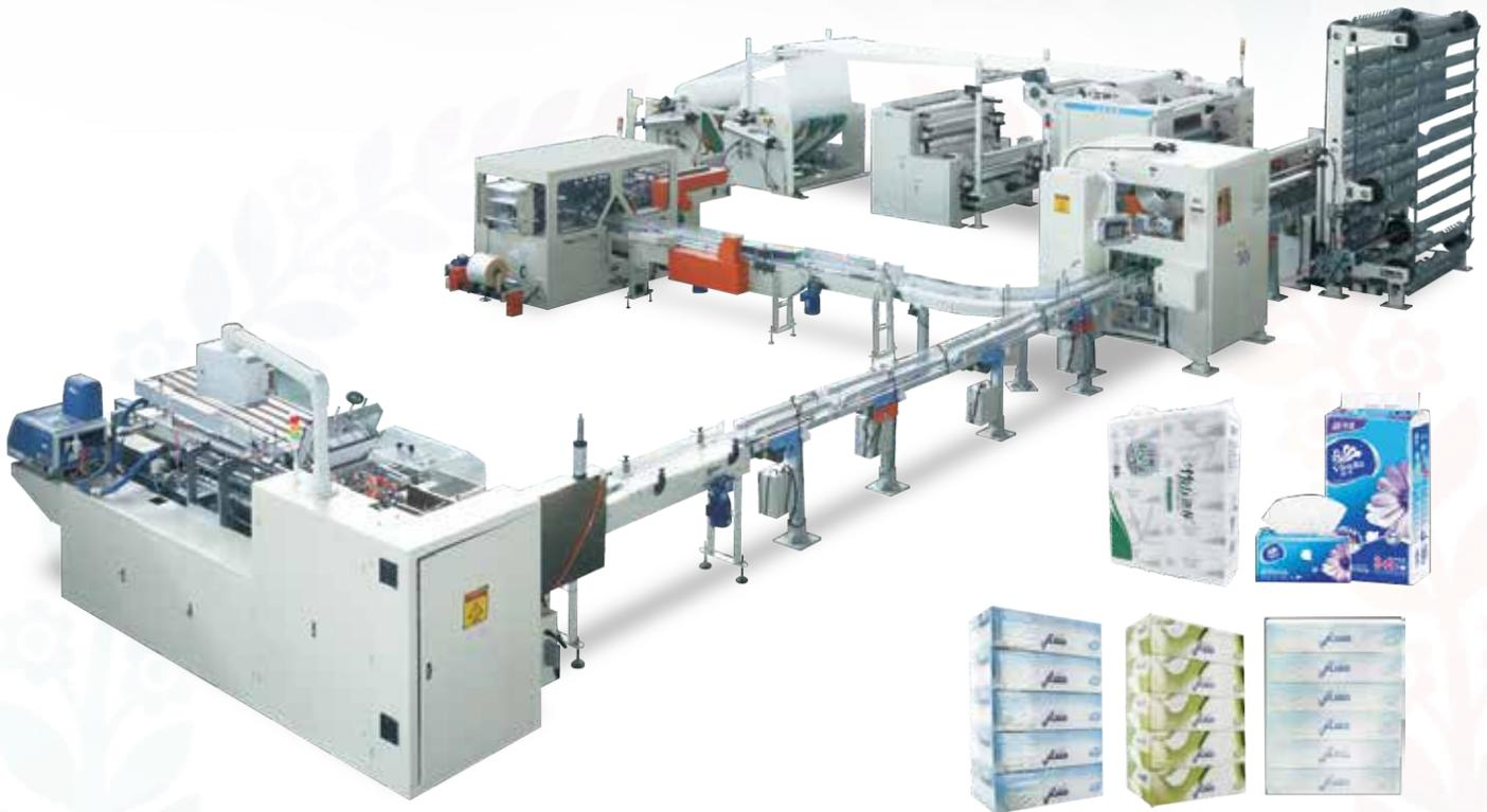
1. High speed-- the working speed is 100m/min or 10-11 logs/min. ( 120 sheets/log)
