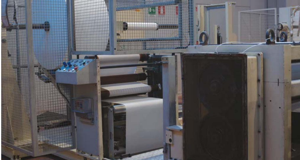
A detail of unwinding and embossing unit of the OMET TV 840 Line in production by Tedim Industry.
