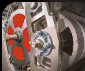
Core turning unit in Panty diaper
