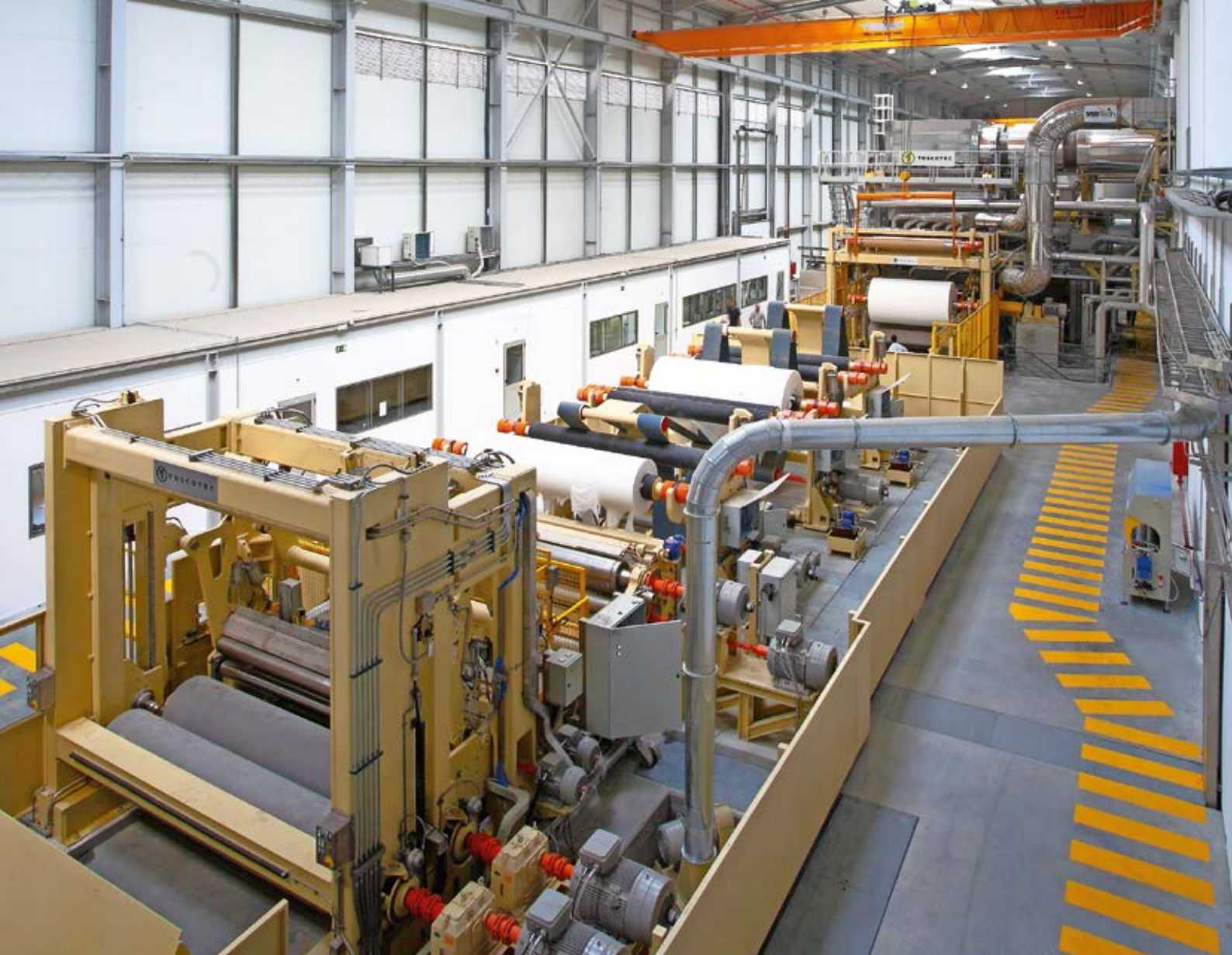
Toscotec TT WIND-H slitter rewinder and AHEAD-2.0S tissue machine at Vila Velha De Ródão mill
