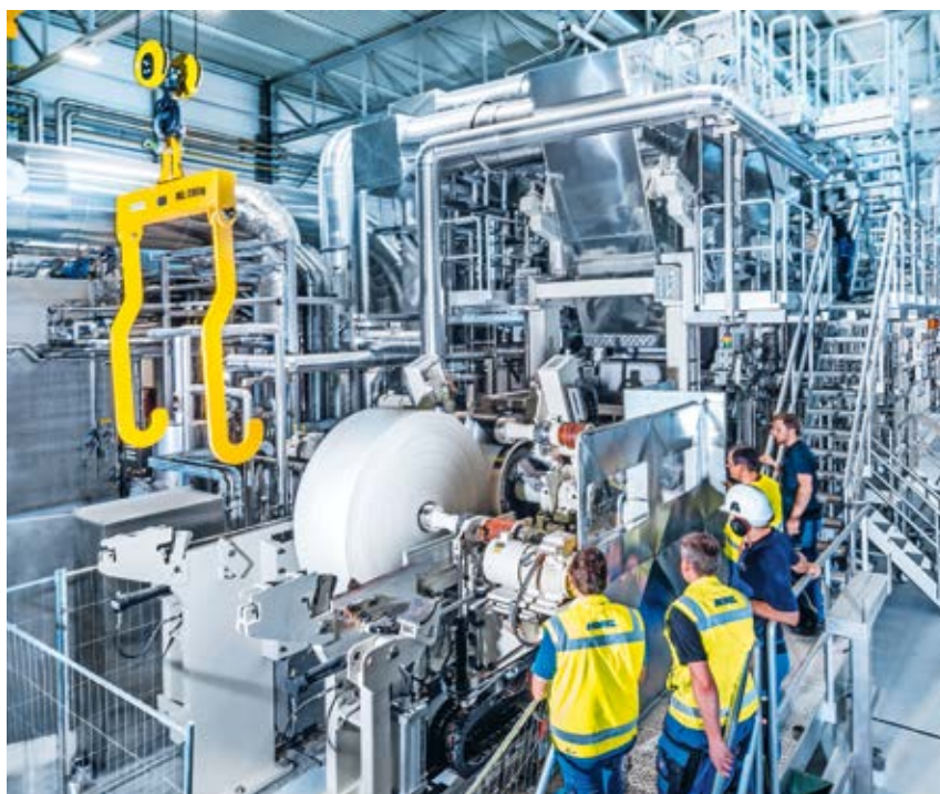
The ANDRITZ tissue pilot plant in Graz, Austria – the PrimeLineTIAC – is currently configured as a PrimeLineTEX machine and offers customers the opportunity to test and develop their future textured tissue. Photo: Andritz
