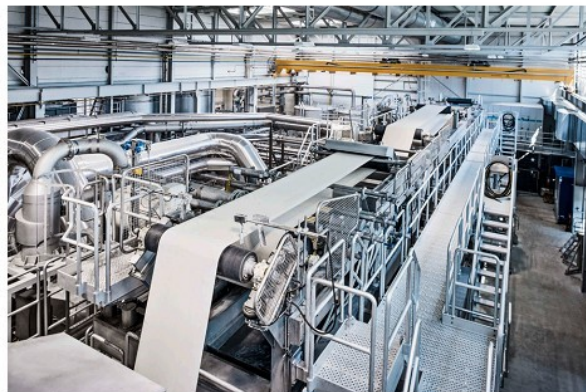
The tissue machine offers various configurations to run trials for the production of conventional, textured, and structured (TAD) tissue.
