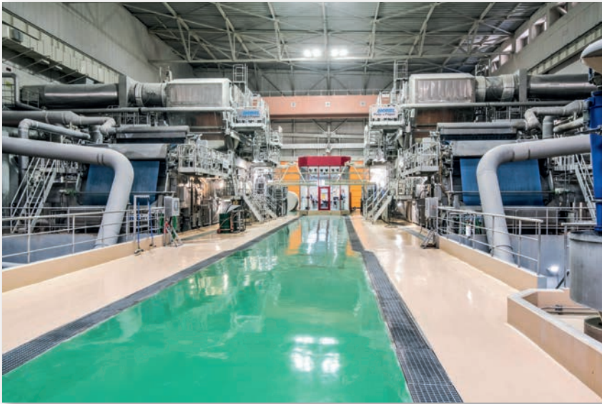
The two identical PrimeLineCOMPACT machines are designed for a speed of 1,800 m/min and for a paper width of 2.8 m.
