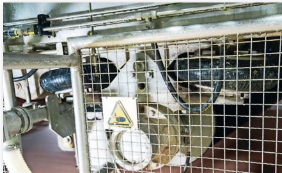
Example of installation: wire and felt guide unit installed in a 1800 m/min tissue machine at Corelex Shin-Ei Paper, Japan.
